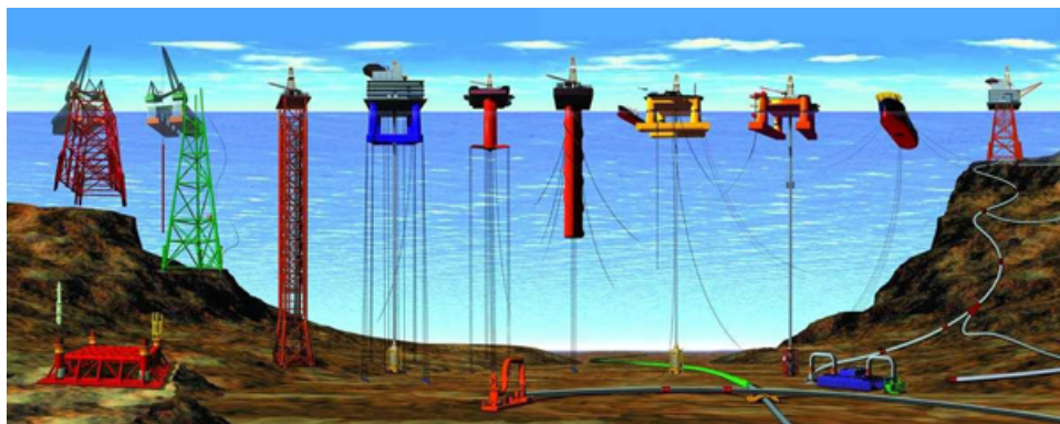
Figure 20: Different types of oil platforms, the majority of the platforms are floating and slowly moving. The picture is from the Office of Ocean Exploration and Research.
