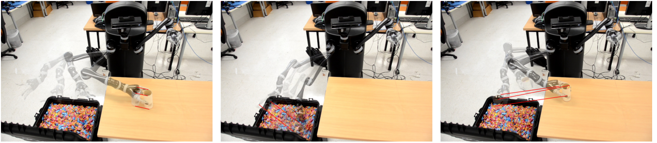
Figure 7: Images showing the robot executing the grasp (left), scoop (middle) and place (right) actions. Red lines track physical features for clarity. In the grasp image, the learned non-prehensile pushing behaviour can be seen at the end of the trajectory.
